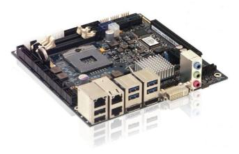
Based on the Mobile 3rd generation Intel® chipset, the motherboard offers an ideal performance-per-watt ratio and the very latest interface technology, e.g. 3<sup>rd</sup> generation PCI Express x16.
