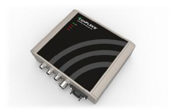
This way, the dissipated power inside the CPU is transferred directly to the enclosure, and there is no need for venting holes or fans.
